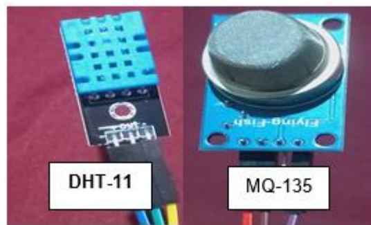
Figure 5. IoT Device for Temperature, Humidity, and Air Quality Sensors
